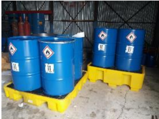
Figure 14: Barrels for used oils stored indoors. The used oils are sent for recycling to the respective Alternative Management System
