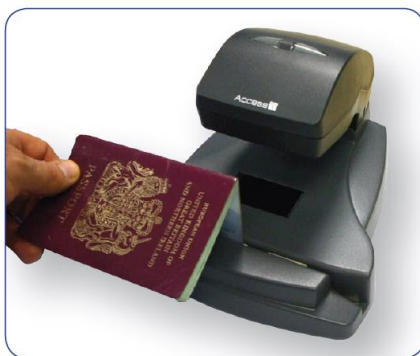
LSR130 OCR option being used to read a passport
